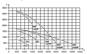
X: airliow m³/h Y: static pressure Pa
